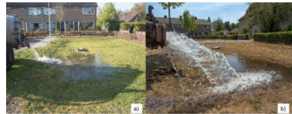
Figure 5. The full-scale infiltration test with a tank truck as water source, was executed repetitively for monitoring the hydraulic behaviour of swales in Dalfsen. a) The swale under normal conditions in 2017. b) The same location after 7 weeks of drought in 2018.
